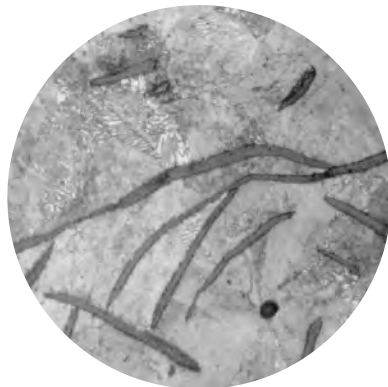
Photomicrograph showing graphite form in gray iron.
