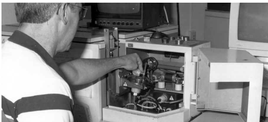
During production, each ladle of ductile iron is checked for exact content of magnesium and other elements with this computer-controlled optical emission spectrometer.
