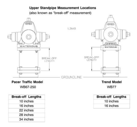
Traffic style fire hydrants are designed so that the upper standpipe and upper operating rod break-off from the lower standpipe and rod when struck by a vehicle, so the upper standpipe is called a "break-off standpipe". Traffic style Pacer and Trend model fire hydrants are supplied with various upper standpipe lengths. Replacement rods must be ordered according to the length of the break-off standpipe.
