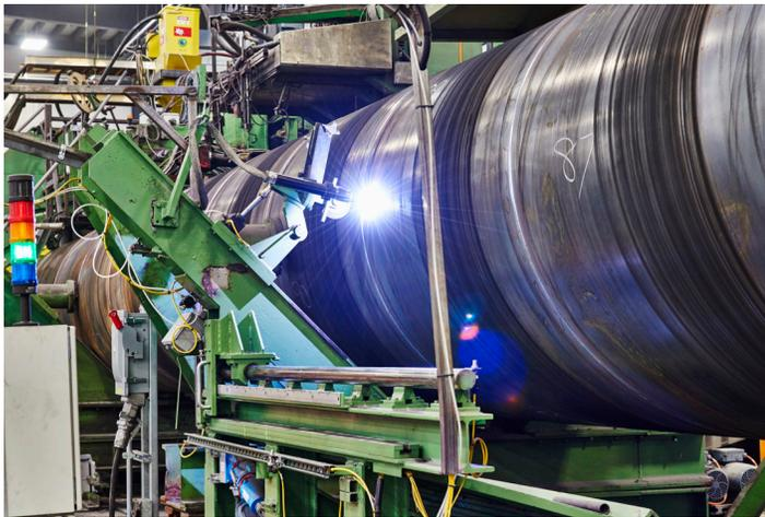
AMERICAN's spiral mills have the capacity to handle coils of steel from 0.1875 inches (4.8 mm) to 1 inch (25.4 mm) in thickness, with yield strengths up to 70,000 psi (482 MPa), to produce high-quality, spiral-welded steel pipe up to 144 inches (3,600 mm) in diameter. This flexibility offers AMERICAN's customers a wide variety of options.
