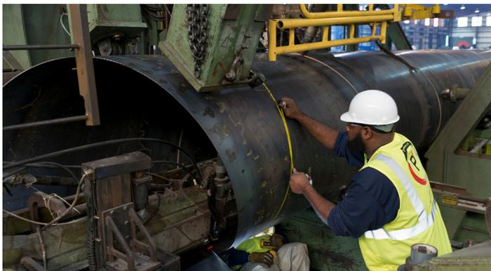
Pipe forming begins when the coils are loaded into the forming section. The steel coil is unwound and fed through the first of four sets of flattening rolls. The flattened coil continues through the forming section that is set at the required angle, based on the diameter of the finished cylinder, and the coil thickness and width.
