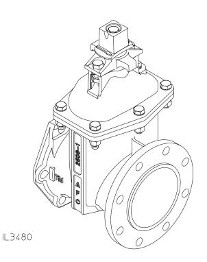
The AMERICAN Series 2500 is available in tapping configurations in sizes 4 in.–48 in. The tapping valve is provided with a rated working pressure of 250 psig and is designed for use in drinking water, sewage, fire protection systems, as well as irrigation systems.
