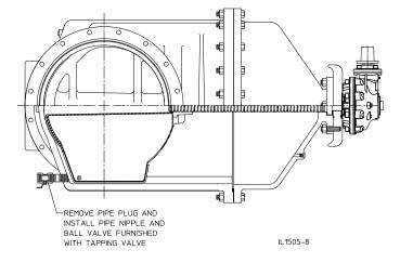
All tapping valves with bevel gears (for horizontal installation) will be furnished with tapped and plugged holes, and a pipe nipple and ball valve for flushing. All tapping valves for vertical installation will have tapped and plugged holes but will not be furnished with pipe nipple and ball valve since flushing should not be necessary for vertical installations.
