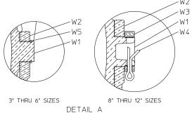
Ref. Description **Material** Cover Gray Iron Α Valve Body В Gray Iron F **Body Seat Ring** Bronze J Cover Gasket Synthetic Fiber with Elastomeric Rubber Hex Head Bolt Stainless Steel K R Hex Nut Stainless Steel S Bumper Rubber Т Rubber O-ring U Bushing **Brass** ٧ Shim Washer **Brass** W1 Disc **Bronze** W2 Arm Bronze W3 Locknut Bronze
