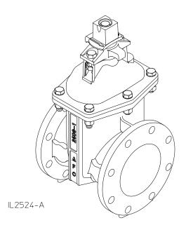
The **Series 2500 Ductile Iron** Resilient Wedge Gate Valve has a rated working pressure of 250 psig and is designed for use in drinking water, sewage, fire protection systems, and irrigation and backflow control systems.
