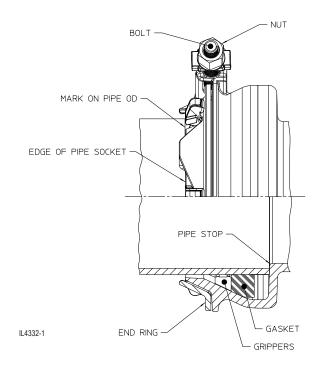
Set the desired pipe deflection angle (4° maximum). ALPHA XL installations on pipe at the top of the OD range may have limited deflection (2° maximum).
