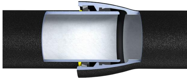
The AMERICAN Field Flex-Ring is a field adaptable restrained joint utilizing a grooved fabricated end in conjunction with a corrosion-resistant, high-strength, low-alloy (HSLA) steel Field Ring. AMERICAN Field Flex-Ring® Restrained Joint Ductile Iron Pipe, utilizing the sealing features of the time-proven Fastite® Joint and a one-bolt restrained connection, provides flexible, easily assembled and positive restraint against endwise separation due to thrust.
