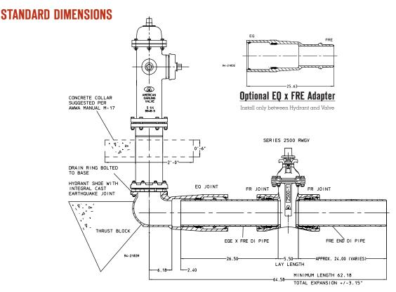
Standard Earthquake Joint Configuration
