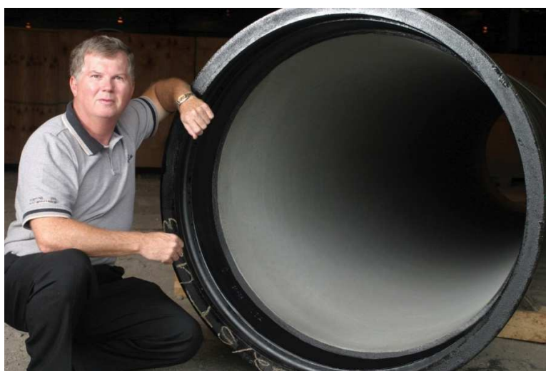
Figure 5. The surface of cement mortar lined ductile iron.
