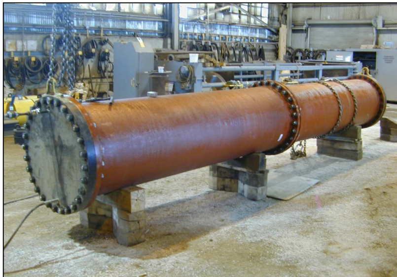
Figure 7: Flange pipe test set up to 500 psi
