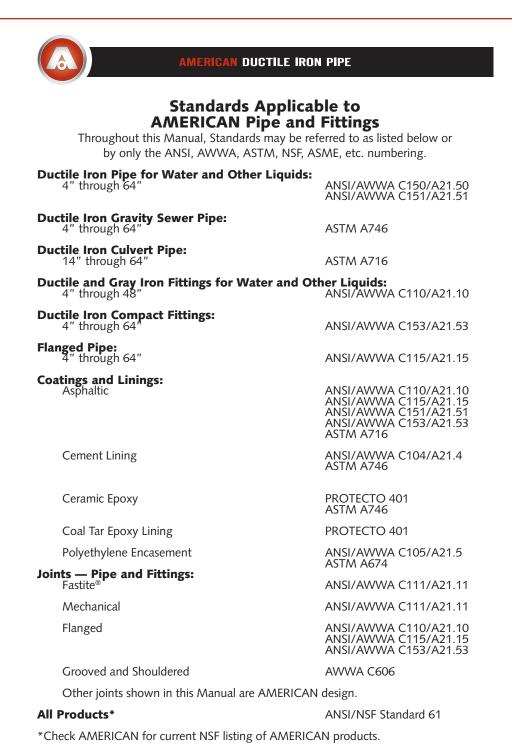
**NOTE:** Many AMERICAN joints, classes of pipe, fittings, and specials are listed by Underwriters Laboratories Inc. and Factory Mutual System. The quality of AMERICAN's products and conformance to appropriate specifications are assured by the British Standards Institute's certification that AMERICAN's quality system complies with ISO 9001 Quality Management System Standard.
