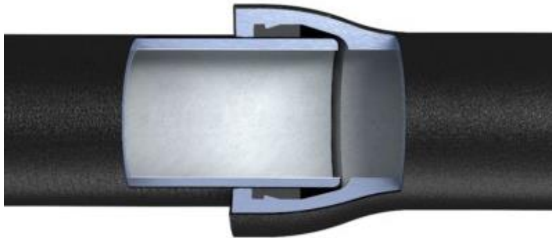
Figure 6. Standard Fastite joint and SBR gasket in straight alignment (American Ductile Iron Pipe 2016).
